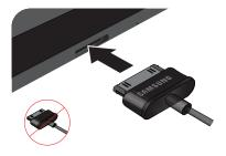
Connect the USB cable to the charging head.
